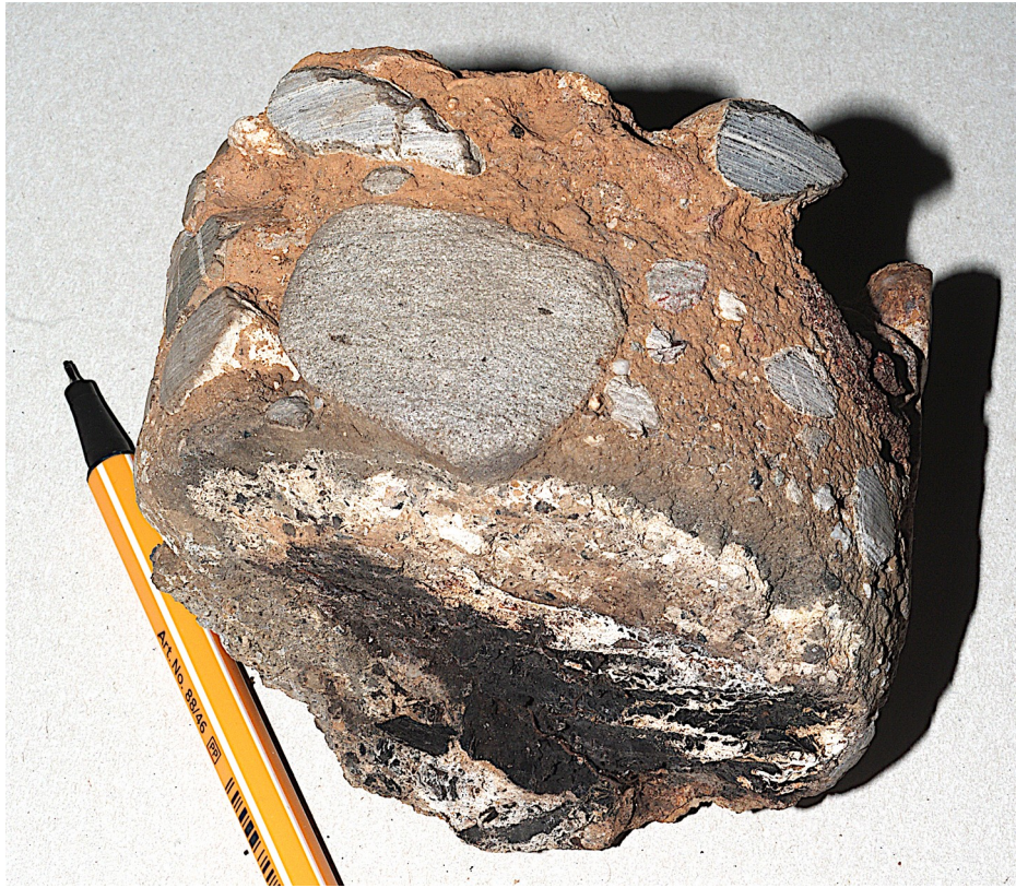
Fig. 13. Drill core from the floor in the center of the #004 crater. As for the trench (Figs. 5, 6), the short core documents the extreme consolidation of the crater subsoil, which is also visible in the ground penetrating radar measurements down to a depth of several meters and is attributed to extreme consolidation and sintering of the clayey-gravel layers. Digging and drilling Gerhard Benske.
