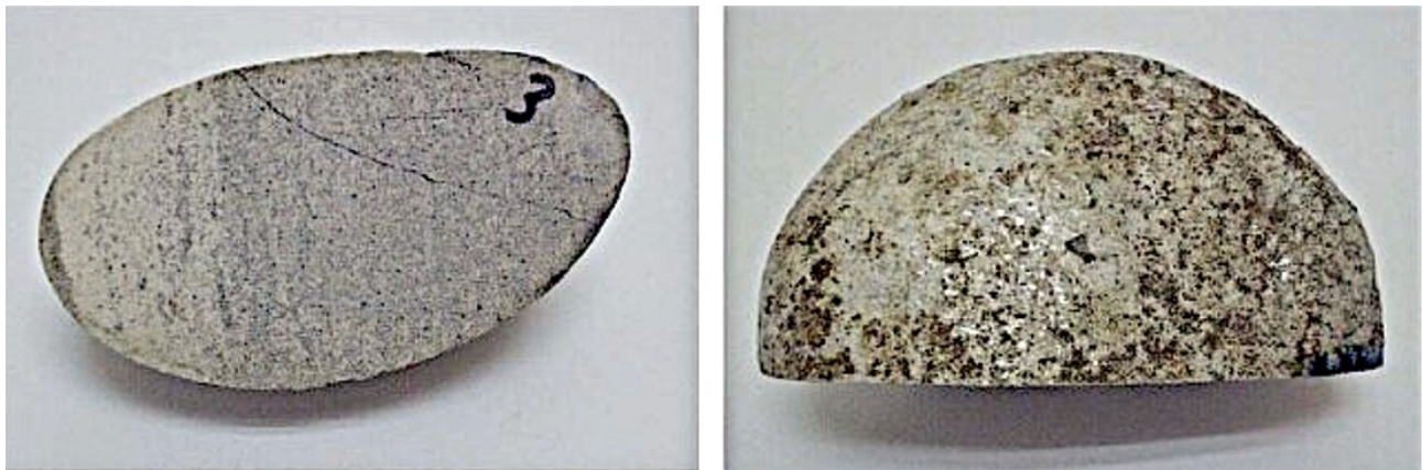
Fig. 18. Quartzite boulder 004-3. Section and surface covered with glass skin.
