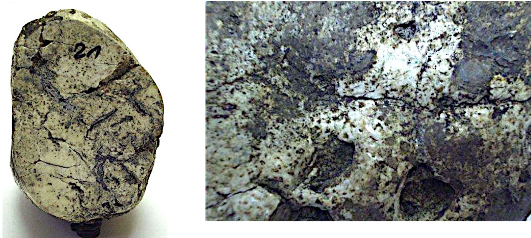
Fig. 33: Quartzite boulder, longitudinal axis 12 cm, remains of a glass crust preserved over a large area on the surface (photo width approx. 2 cm).
