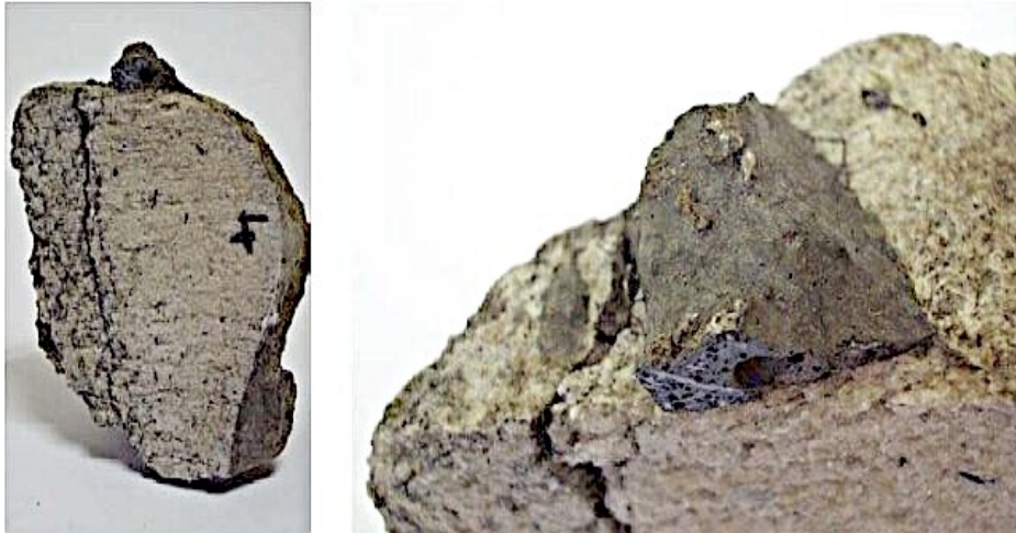
Fig. 19. Sample 004-4: incision and fusion patina on residues of vitreous coating.
