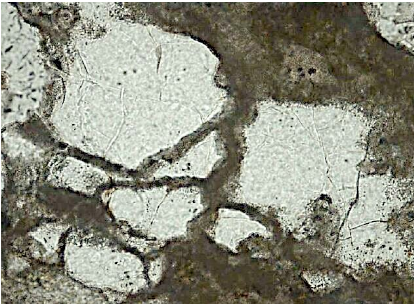
Fig. 28. Quartz grains cracked due to spallation, longitudinal edges of the photos ~ 0.8 mm. The spallation cracks are filled with recrystallized glass.
