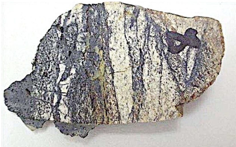
Fig. 24. Section of sample 004-8. longitudinal axis 6 cm. Inhomogeneous, light-dark
